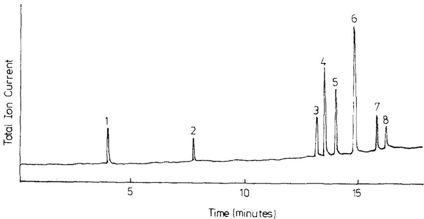
FIG. 2. Chromatogram of the volatile components in the mandibular gland secretion of a single *M. nortoni* female. GC column was 50 m OV-101, fused silica, programmed from 70° to 200°C at 4°/min. Peak numbers are referred to in the text and Table 1.
