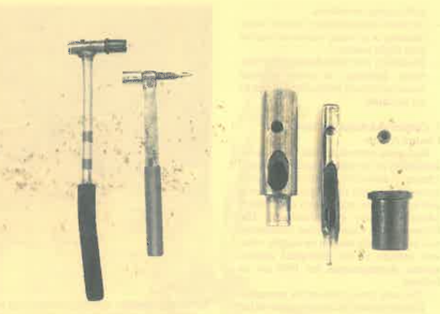
a) SWAT inoculation hammer (top) and Gould punch (bottom). b) disassembled SWAT hammer; hammer head, wad punch, allen screw, and rebound rubber.
