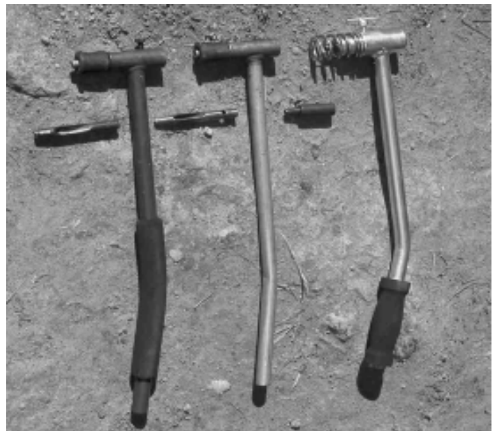
Inoculation hammers. From left to right: South African designed hammer used in 2004, Australian designed hammer, new South African designed hammer used in 2005
